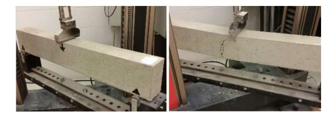
Pic. 3. Beam before and after testing
