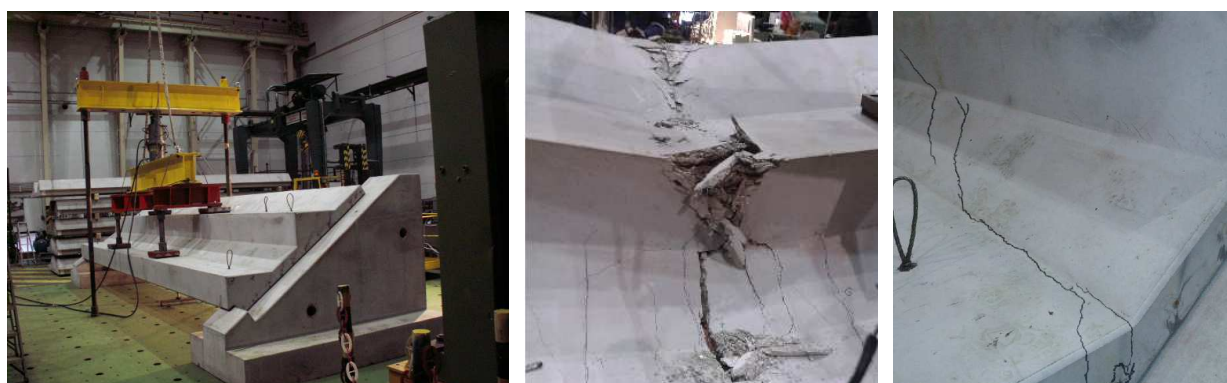
Fig.5. a. Laboratory tests b. Compressed zone c. Shear
