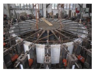
Fig. 1: Geometry and loading configuration of the tunnel
