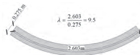
Figure 2: An example of a segment aspect ratio \lambda .
