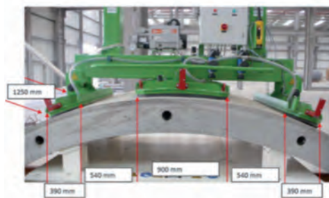
Figure 21: Vacuum lifting system
