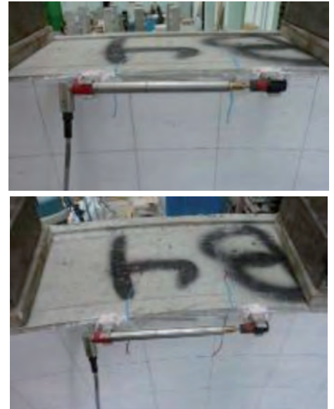
Figure 19: Point load test: a) first cracks (1650 kN) b) crack pattern at load level of 2000 kN
