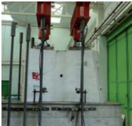
Figure 18: Point load test set-up
