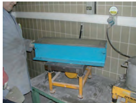
Figure 39: Vibrating an EN14651 beam
