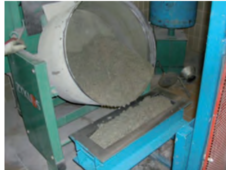
Figure 38: Filling the mould of an EN14651 beam
