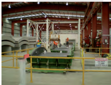
Figure 23: Segment production factory with carousel plant and segment pre-storage
