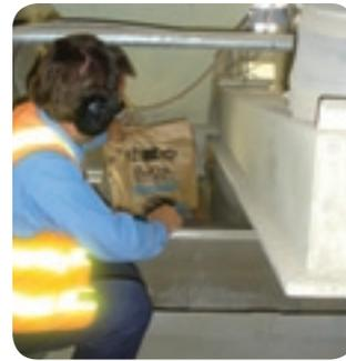
Adding Barchip fibre directly into load chute.
